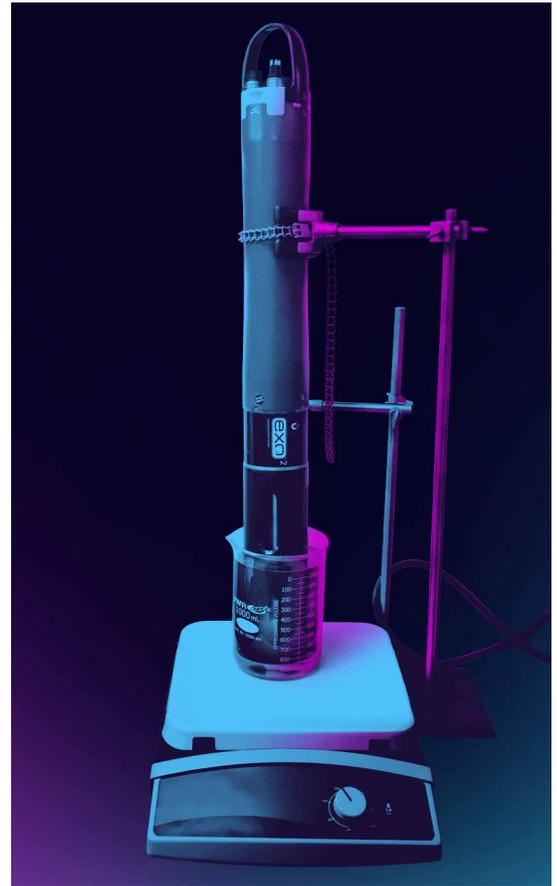
While the sensor LED values are stabilizing, verify that there are no bubbles accumulating on the sensor faces of the NitraLED or turbidity sensors. Be sure to watch the turbidity values for stabilization as well. If turbidity continually rises over time, this is most likely due to bubbles accumulating on the sensor face. Even the smallest bubbles can have an impact on sensor readings; if there are bubbles, remove the sonde from the water briefly and reinstall.
